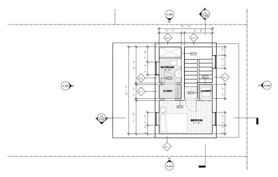
Fig 3.5 Second Floor Plan As-Built
