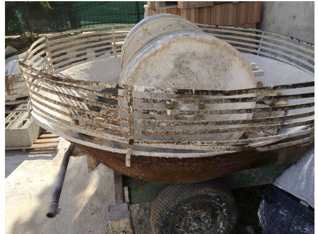
Fig 1.12 Crushing hemp and line blocks for reuse
