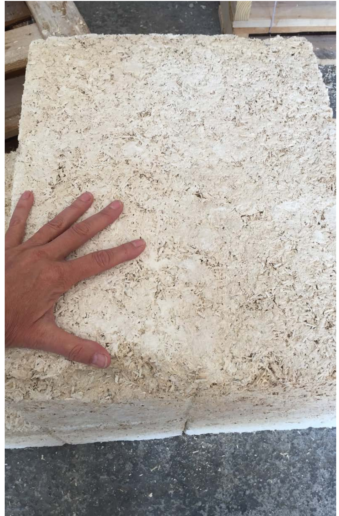
Fig 5.1 Hempcrete Block at Pedone Architects Materials Yard
