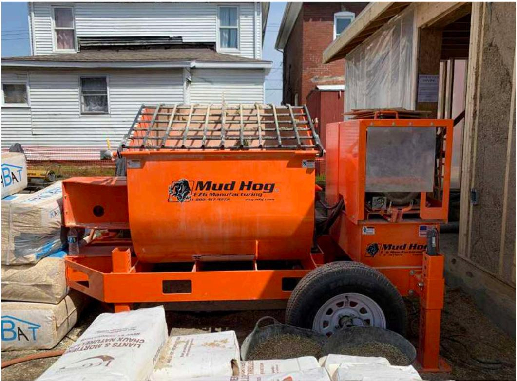
**Fig 5.7** The install starts with the Mud Hog, which mixes the hemp hurd, lime and water
