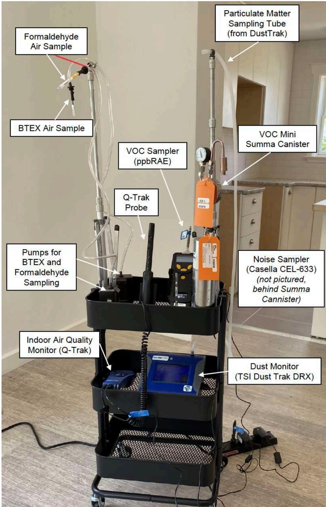
Fig 8.3 The sampling station all set up
