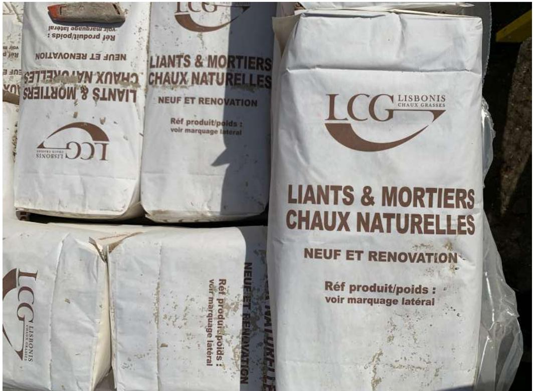
Fig 5.4 Bags of Lime imported from France to mix with the Hemp hurd
