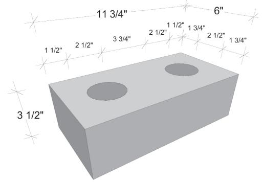
Size: 6" x 11-3/4" x 3-1/2" (height can vary from 2" to 5") Weight: 15.85 lbs average Compressive Strength: 1250 psi average Modulus of Rupture: 305 psi average Dry Density: 161.7 pcf average (normal weight) Thermal Conductivity: 0.35 W/mK R: 0.42/in or 2.52 for 6" wide block
